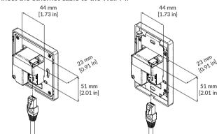
4. Click off the front panel. Screw the Wall-M unit into the electrical box.
